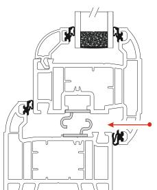
**STAY GUARD ELITE SG036** on outer frame and sash for all types of stays to include Egress/Easy Clean
